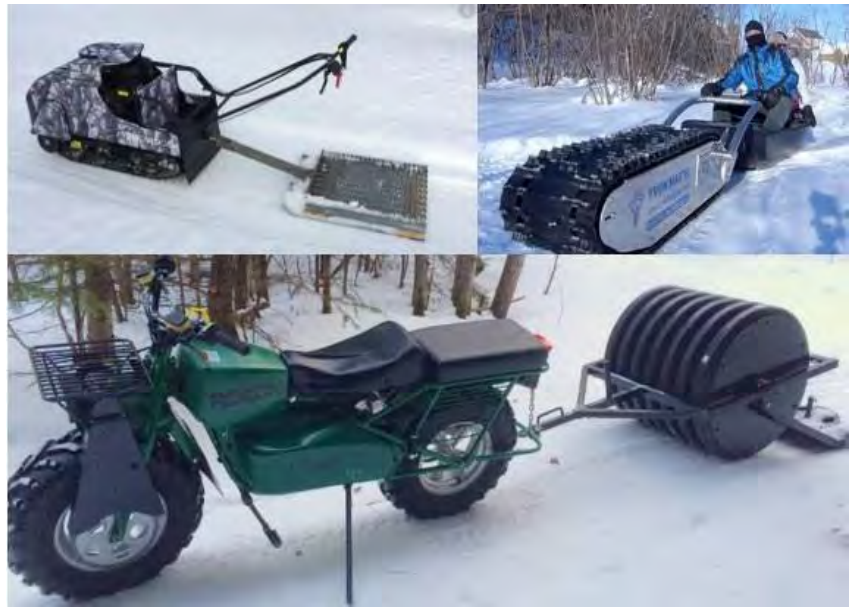
Figure 9. From top left; A SnowDog; Yvon Martel's MTT-136 electric snow machine; and a Rokon, a two-wheel drive motor bike.
